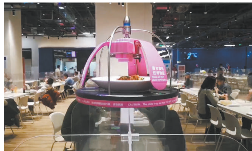
Robot serves food from ceiling in the medium dining hall at Beijing 2022 to minimize contact. (PHOTO: S&T DAILY)
